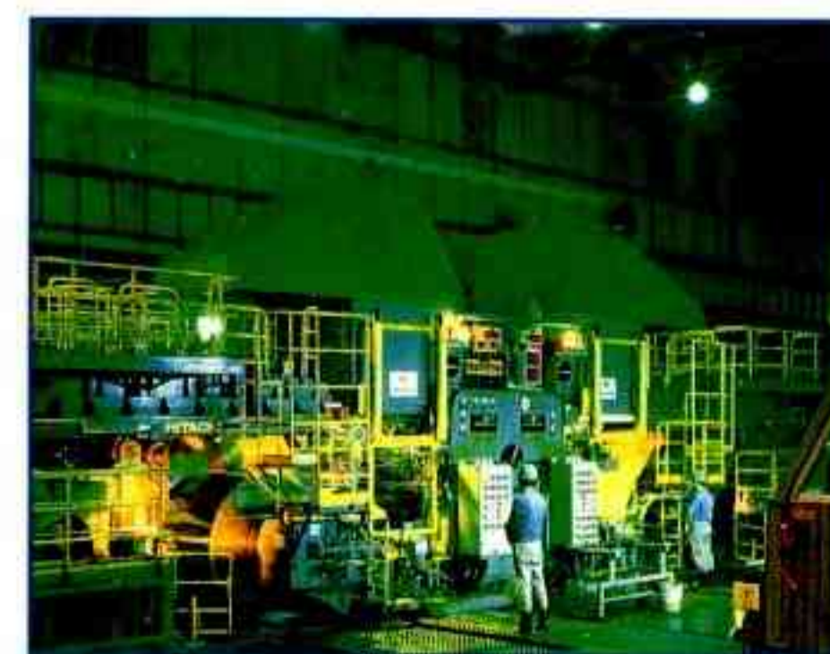
冷間圧延機/Cold strip mill
