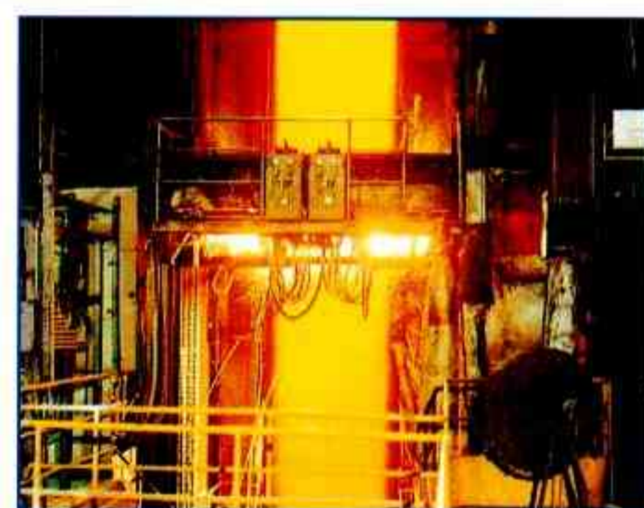
連続铸造機/Continuous casting machine
