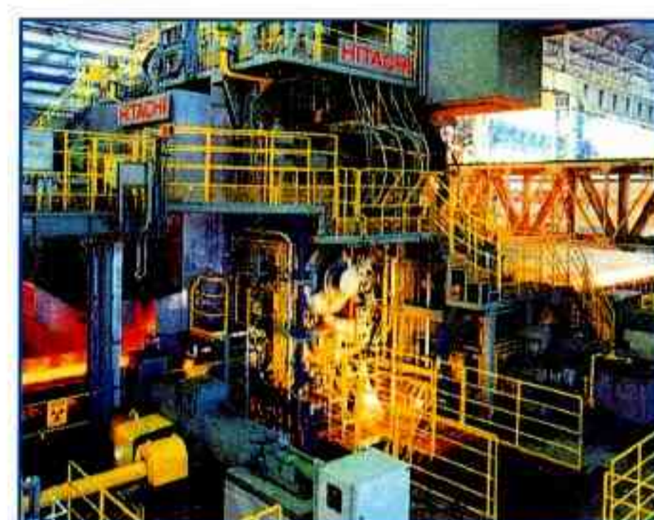
熱間粗圧延機/Hot rolled roughing mill
